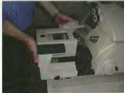
Fig. 3.21: Mounting the FC6 cryochamber on the Ultracut UC6.
