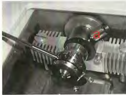
Fig. 4.1: Inserting the cryo specimen holder before locking it with the torque limited screw (a).
