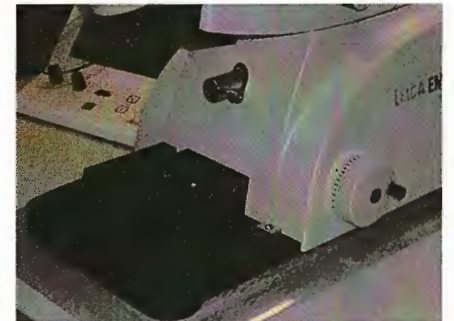
Fig. 3.10: Ultracut UC6 after removal of armrest, knife support and segment arc.
