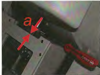
Fig. 3.22: The cryo specimen arm (a) has been guided onto the specimen arm of the UC6.
