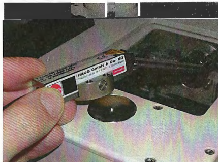
Fig. 3.34: Antistatic electrode with holder on cryochamber.
