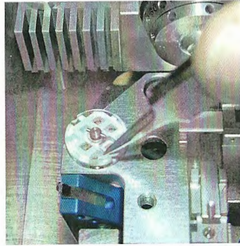
Fig. 5.16: Transfer grid into the transfer container.
