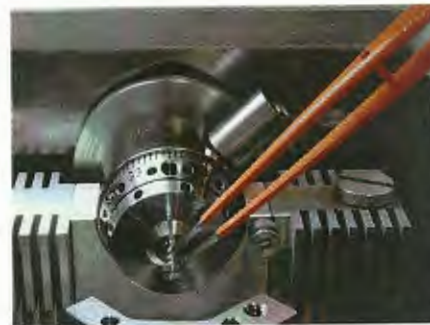
Fig. 4.9: Inserting the specimen pin with the insulated forceps.
