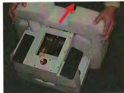
Fig. 3.18: Removing foam packaging from FC6.
