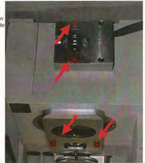
Fig. 3.19: Transport locking screws on FC6 rear side and bottom.
