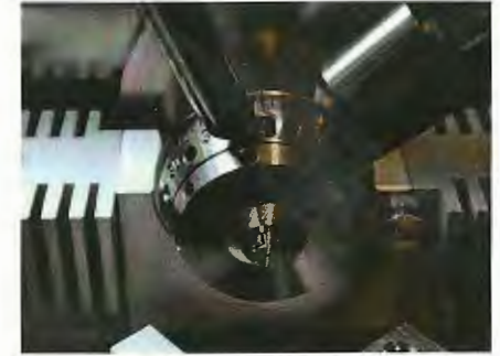
Fig. 4.10: Locking the specimen pin in the cryo specimen holder. Arrows indicate the direction of the force applied for locking.
