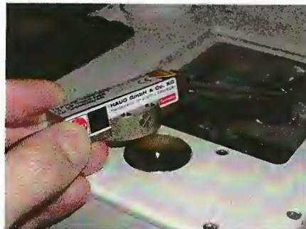
Fig. 3.2: Antistatic Electrode in holder, both supplied with the EM FC6.
