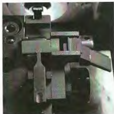
Fig. 5.11: Grid ready to be pressed.
