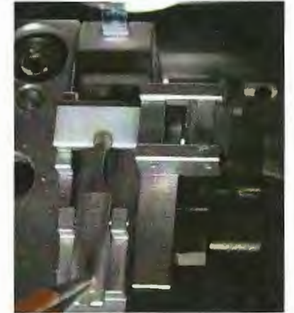
Fig. 5.7: Clamping grid in grid holder.
