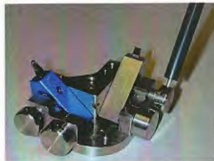
Fig. 4.3: Locking the knives, here showing a Diatome diamond trimming tool and a Diatome 35° cryo immuno knife.
