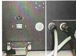
Fig. 3.33: Touch screen control unit, rear side with remote control cable of antistatic device connected.
